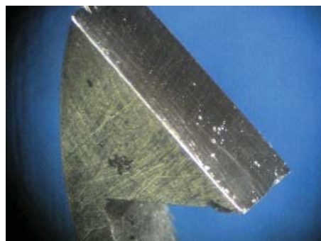
An entry pallet. After welding, the surface was so hard I could only dress it with a diamond file. By depositing metal on the sharp edge of the discharge corner of the pallet I was able to reduce the inside drop to a more acceptable level.
