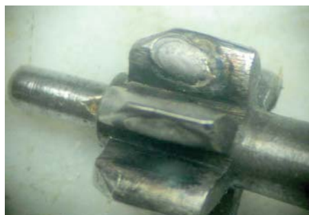
Left: Worn pinion leaf. Middle: Welded pinion. Right: Pinion worn more than half way through, one leaf is partly welded.
