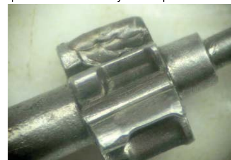
Left: Worn pinion leaf. Middle: Welded pinion. Right: Pinion worn more than half way through, one leaf is partly welded.
